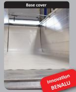
Base cover equipment designed to ease the flow of products that are sticky and ensure total safety (Patent no. FR2976532)
