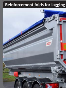
Folds on the sides which allow the entire box to be stiffened.
