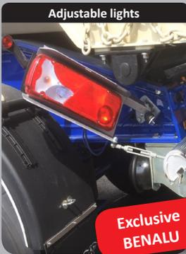
Movable headlamp fittings that are adjusted when adjusting the underide guard. Optimisation of the protection of the lights to the finisher!
