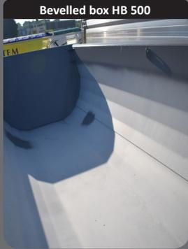
Steel box HB 500 with sides that are rounded by bevelled folds which improve run-off and greater rigidity.
