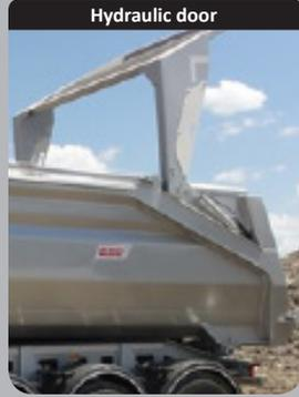
Single- or double-acting hydraulic door with a large opening angle of 95°.
