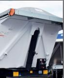
Jack with a lug firmed fastened which guarantees robustness suitable for building and public works.
