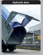
Single- or double-acting hydraulic door with a large opening angle.
