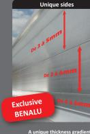
A unique thickness gradient! The "double skin" technology allows the internal thickness to be varied over the height of the vehicle.
